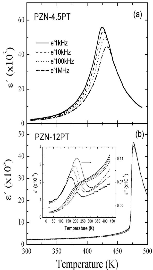
**Figure 2.** Temperature dependence of the dielectric permittivity in PZN-xPT crystals along the cubic  $[001]$  direction.
