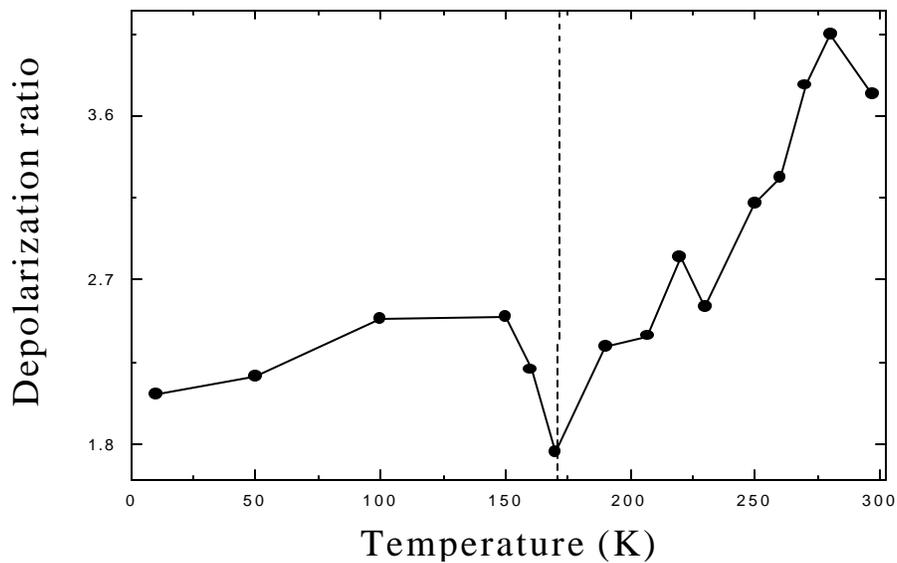
**Figure 4.** Depolarization ratio of the  $780\text{ cm}^{-1}$  band of PZN-12PT as a function of the temperature.
