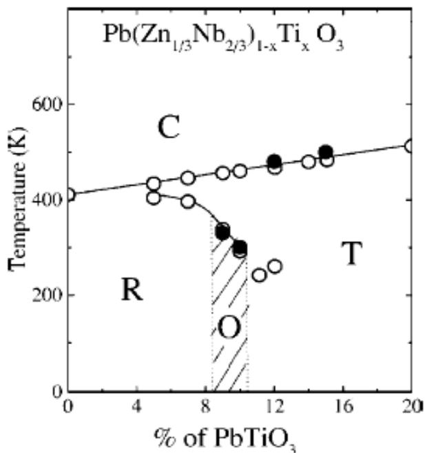
Figure 1. Phase diagram of PZN-xPT relaxor ferroelectric around the MPB according Reference [2].
