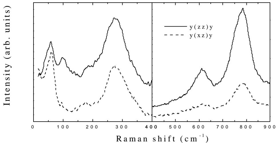
**Figure 3.** Raman spectra of PZN-12PT at room temperature in the  $y(zz)y$  and  $y(xz)y$  scattering geometries.
