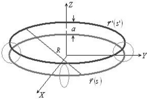
**Figure 5.** Circular loop antenna and its associated vectors.
