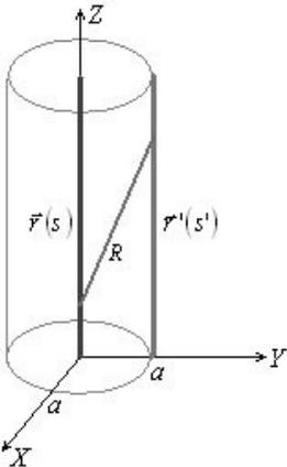
**Figure 3.** Dipole antenna and its associated vectors.
