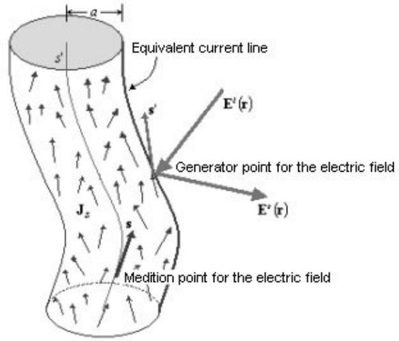
Figure 2. Unit tangential vectors for the thin wire.
