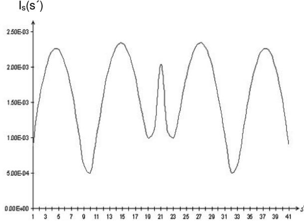
**Figure 4.** Current distribution for a  $2\lambda$  length dipole antenna.
