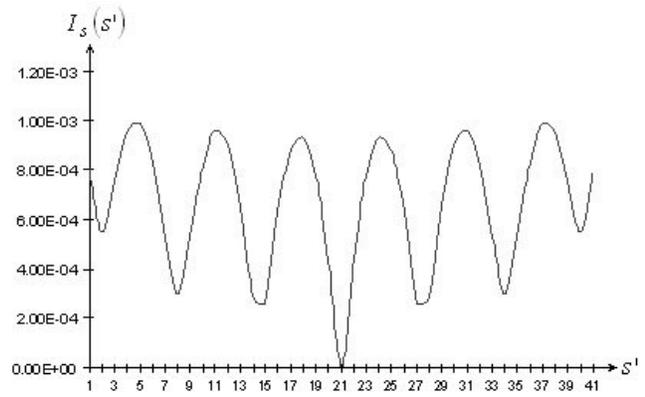
**Figure 6.** Current distribution for a  $3\lambda$  length circumference loop antenna.
