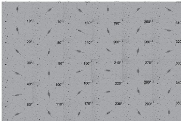
Figura 2: From top to bottom and left to right: Optical micro-scropy images showing the orientation of a micro-crystal upon rotation of the linear polarization of the trapping beam. The rotation angle of the  $\lambda/2$  retardation plate is indicated.
