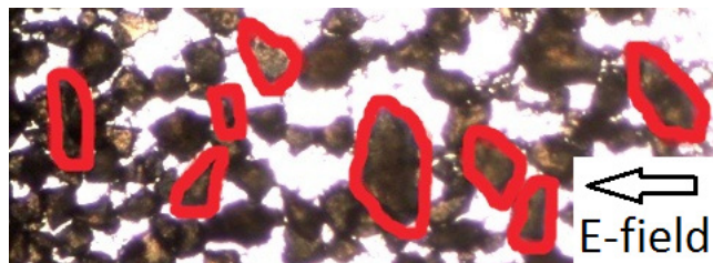
Figure 8: High concentration of laponite particle aggregates between two electrodes with an AC E -field of 500 \text{ V/mm} applied. Several particle aggregates (red-color-marked) were not able to re-orient fully with their longest axis along the E -field lines due to jamming. This will effectively lower the value of the nematic order parameter.
