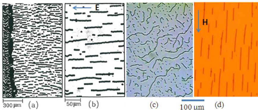
Figure 1: (a) and (b) Electric alignment of 5  $\mu m$  polystyrene spheres in water at field frequency  $f = 1$  kHz and  $E = 5$  V/mm. (c) Permanent magnetic microbeads in a very weak in-plane magnetic field. (d) Alignment of 4  $\mu m$  polystyrene microspheres in a ferrofluid.
