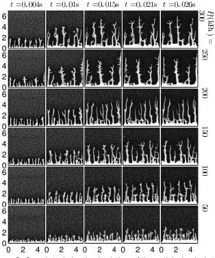
Figure 2: Snapshots during the simulations of the particle density in the Hele-Shaw cell, displayed for decreasing injection pressure  $P_{_I}$  from top to bottom and as a function of time (left to right). Low particle density appears brighter in the snapshots. Under air injection, fractures, fingers and dispersed bubbles of low particle density emerge and propagate. x- and y-axis units are given in cm. The y-axis specifies the distance from the inlet.
