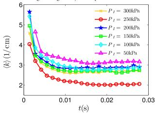
Figure 6: The average of the spatial finger wavenumber in x direction.
