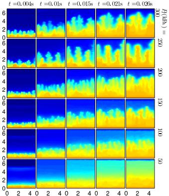
Figure 3: The pressure evolution for decreasing injection pressure  $P_{\scriptscriptstyle I}$  (top to bottom) and as a function of time (left to right). High pressure appears yellow (brighter) in the snapshots. x- and y-axis units are given in cm.
