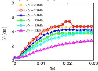
Figure 4: The position of the most advanced finger/fracture as a function of time at different injection pressure  $P_{_{I^{\ast}}}$ . The higher the injection pressure  $P_{_{I}}$  the further fingers grow.
