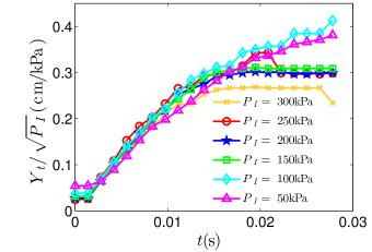
Figure 5: The position of the most advanced finger/fracture rescaled by the square root of the injection pressure  $\sqrt{P_I}$ . As a function of time the graphs at different injection pressure  $P_I$  collapse onto a single graph.
