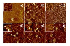
Figure 1. AFM images of seed layers annealed at a) 250°C, b) 300°C, c) 350°C, d) 400°C, e) 450°C and f) 500°C on top of glass substrates. The large images have scan dimensions of 1  $\mu m$  and the insets have scan dimensions of 125 nm.
