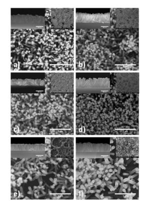
Figure 2: SEM images of ZnO nanorods grown on seed layers on glass annealed at a)  $250^{\circ}$ C, b)  $300^{\circ}$ C, c)  $350^{\circ}$ C, d)  $400^{\circ}$ C, e)  $450^{\circ}$ C and f)  $500^{\circ}$ C. On the insets transversal and magnified view.
