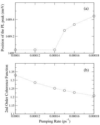
Figure 1: Uniform pumping. (a) Position of the PL line as a function of the pumping rate. (b) Photon second-order coherence function.
