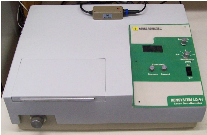
Figure 1. LD-01 laser densitometer. Note the USB external module over the instrument.
