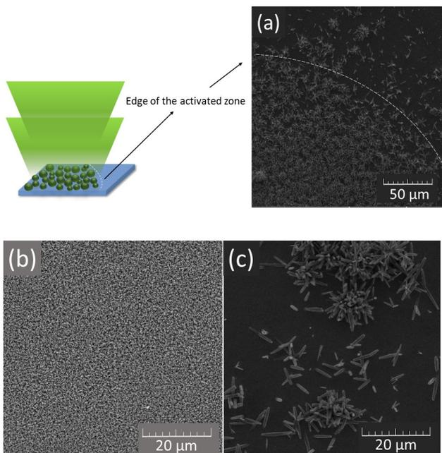
Figure 3. SEM images show: (a) edge of the laser spot (6 pulses), (b) homogeneous nanorods growth inside the laser spot (2 pulses) and (c) disordered growth outside the laser spot (2 pulses). The images scales are (a) 50  $\mu\text{m}$ , (b) and (c) 20  $\mu\text{m}$ .
