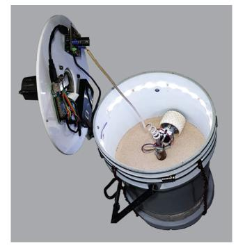
Figure 1. Lab-in-a-bucket: photograph of the accelerated laboratory. When attached to a 15-m long Atwood machine, the wheel can "feel" an effective gravity equivalent to that on the surface of Mars.
