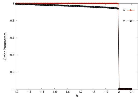
Figure 9. Order parameters as a function of  $h$  for  $T = 0.05$ . A discontinuous transition is observed for both of the parameters. So, the transition from stripes to paramagnetic phase is direct.
