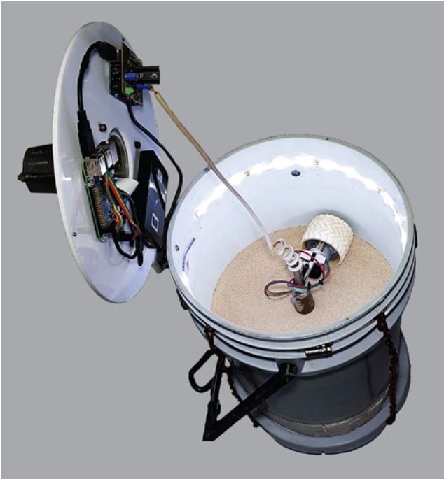
Figure 1. Lab-in-a-bucket: photograph of the accelerated laboratory. When attached to a 15-m long Atwood machine, the wheel can "feel" an effective gravity equivalent to that on the surface of Mars.
