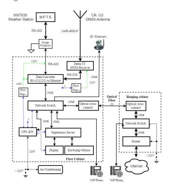
Figure 1. Block diagram of the equipment of the Russian-Cuban co-located station.
