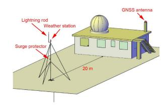
Figure 6. GNSS antenna and weather station layout.
