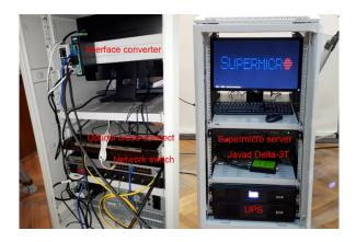
Figure 3. Laboratory assembly of equipment of the Russian-Cuban co-located station (Floor cabinet).
