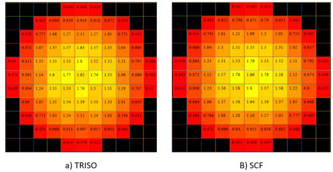
Figure 8. Radial power distributions at BOL state.
