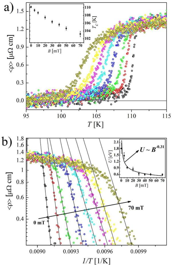
Figure 2: (a) Resistive transitions of a Bi-2223/Ag transverse bridge for different values of the applied magnetic field ( $B = 0, 5, 10, 20, 30, 40, 50$  and  $70$  mT from right to left). The inset shows the dependence of the critical temperature with the applied magnetic field. (b) Arrhenius plot of the data shown in Fig. 2(a). The dependence of the activation energy with the applied magnetic field is shown in the inset.
