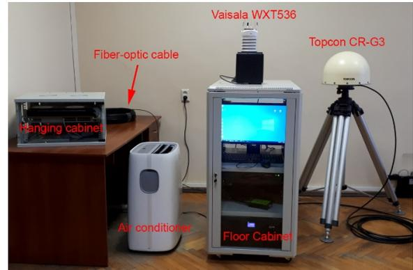
Figure 2. Laboratory assembly of equipment of the Russian-Cuban co-located station (general view).
