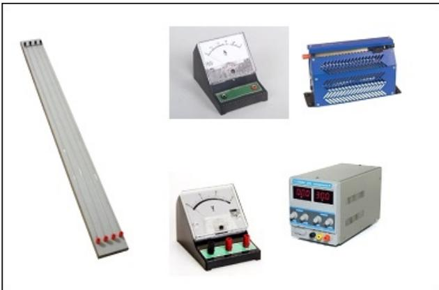
Figura 1. Equipment for a traditional experiment about Ohm's law.
