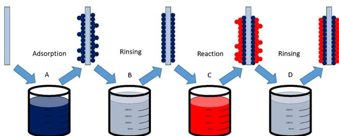
Figure 1. Diagram of one SILAR cycle. In step A the anions of the precursor solution are adsorbed by the substrate. During steps B and D the sample is rising in a solvent to eliminate not strongly attached ions. The last step involves immersing the substrate into reaction solution C to form the thin film.
