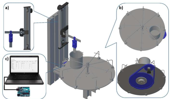
Figure 2. Representation of the system and each subsystem: a) Mechanism responsible for immersing the substrates in the precursor solution. b) Acrylic platform that holds the beakers containing the precursor solution to be used. c) Control unit that enables communication between the computer and the device.
