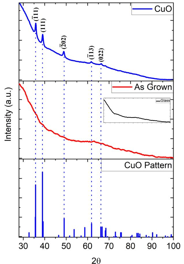
Figure 7. X ray diffractograms of the substrate, as grown, and  $CuO$  samples.
