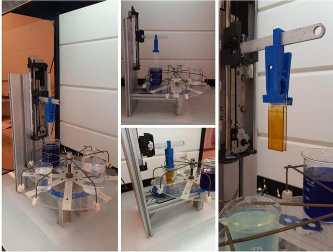
Figure 6. Collage of images of the system during a deposition procedure.
