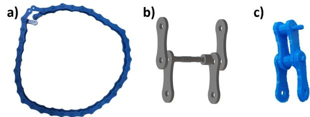
Figure 4. Representation and images of a link in the chain. a) Photo of the printed chain. b) Design of a link to form the entire chain. c) Photo of a printed link.
