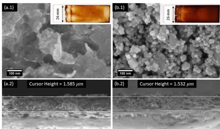
Figure 8. Top-view (a.1) and cross-sectional (a.2) SEM images of the as grown sample. Top-view (b.1) and cross-sectional (b.2) SEM images of the CuO sample. Each top-view SEM image includes an inset photo of the sample.
