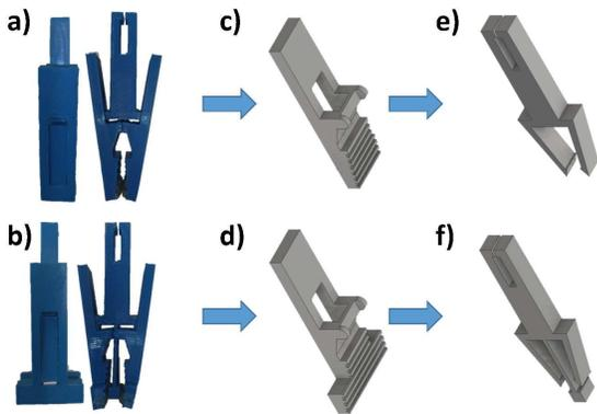
Figure 3. Representation and images of the sample holder. Photos of the two functional clip versions (a,b). Arms of the clip (c,d). Piece that provides closing pressure (e,f).
