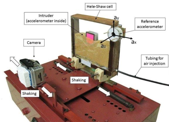
Figure 1. Experimental setup for quasi-2D measurements. Both the Hele-Shaw cell and the camera are synchronously shaken in the lateral direction. Accelerometers attached to the Hele-Shaw cell and the intruder bring the key information to quantify the sinking dynamics
